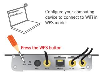
The WPS function will automatically set up a secure connection between your router and computer
